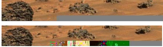
Figure 8 An example of an image corruption which can be revealed by decoding sectors one at the time.
